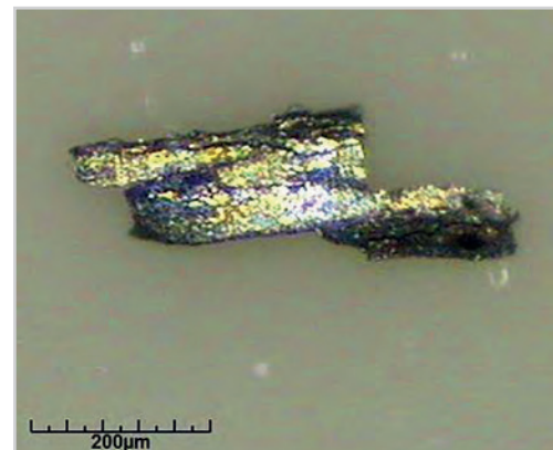
Metal particle from screw thread
